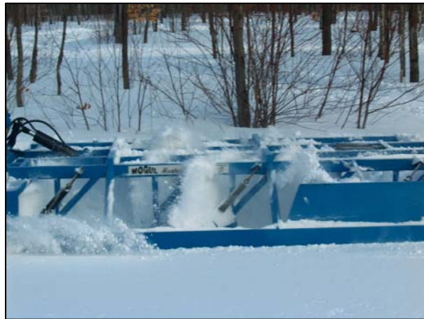
Photo 4.5 Keep processed snow inside the drag!
