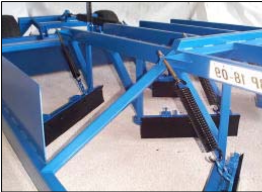
Photo 2.7 Beveled cutting blades
