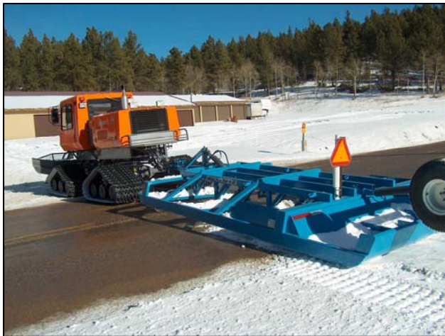
Photo 4.8 Always raise the drag to cross roads
