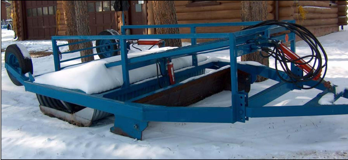
Photo 2.18 Typical single blade drag
