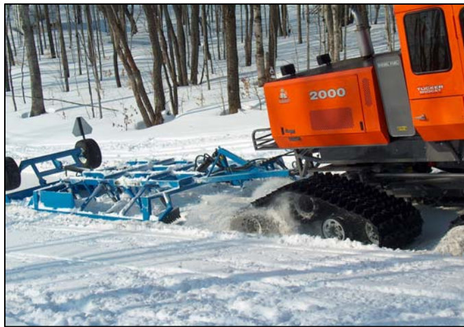
Photo 4.13 Beware of trenches dug by spinning tracks
