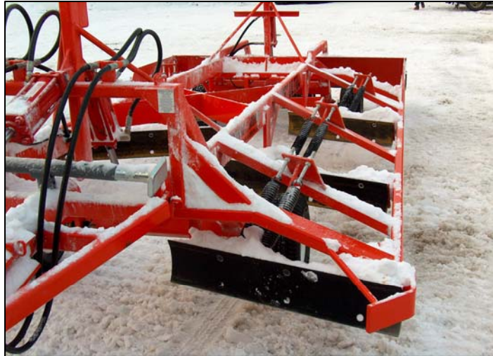
Photo 2.1 Typical multi-blade drag
