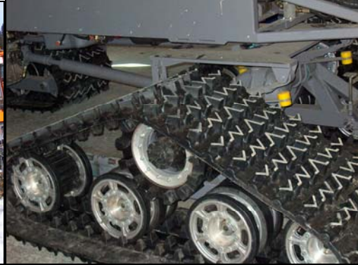
Photo 2.27 Example of rubber track
