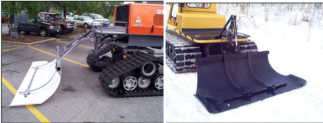
Photo 2.24 Typical compactor bars
