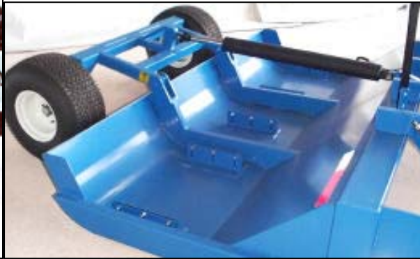
Photo 2.12 Radius lip on rear of pan
